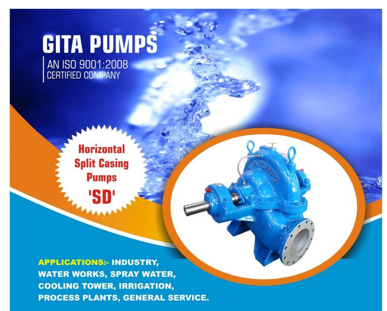
**DESIGN FEATURES:** Gita make 'SD' pumps are horizontal split casing, horizontal shaft pumps with double suction impeller. Suction and delivery branches are cast integral with lower half casing. Inspection is easy and quick by removing upper casing and rotor assembly.
