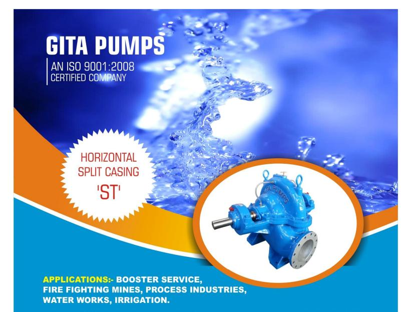
**DESIGN FEATURES:-** Gita make ST pump are horizontal split casing, horizontal saft, two stage centrifugal pumps, They employ two single entry closed impellers, mounted on shaft with suction in opposite direction. This arrangement balances the end thrust hydraulically..
